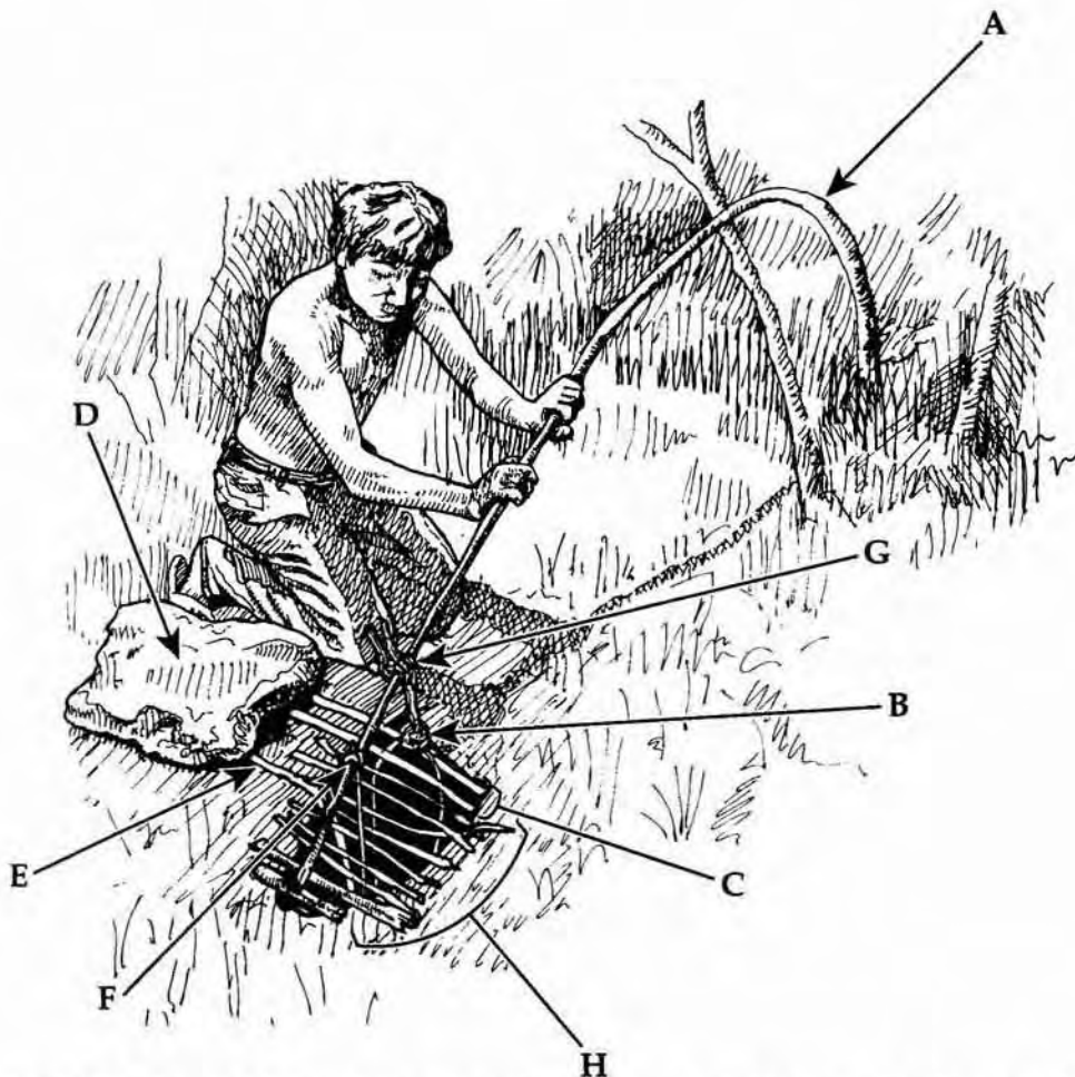
FIGURE 4.— View of the gopher snare trap before a covering of leaves and soil is applied. The fundamental components of the trap include: (A) the spring sapling, (B) the bark strip attached to the wire snare, (C) the two parallel shafts which are embedded into the sidewall and flank the snare, (D) The stone used to anchor the free ends of the parallel shafts and the bait vine shaft, (E) the shaft that anchors the bait vine to the floor of the borrow, (F) the bait vine attached to the spring sapling, and (G) the bark strip attached to the spring sapling. From this perspective, the gopher will approach the trap from the upper right-hand corner of the illustration (drawing by Charles Bouscaren).
