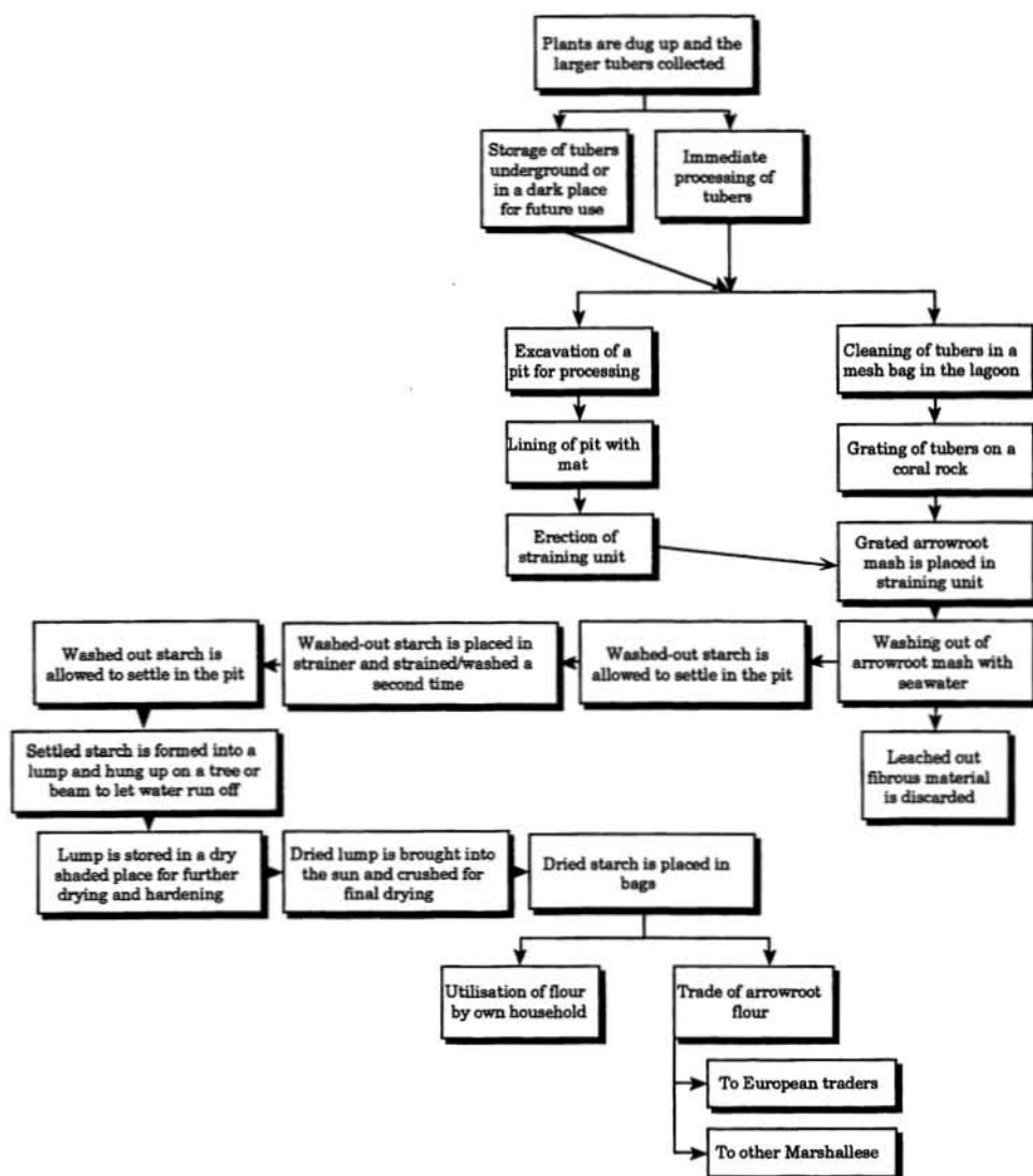
FIG. 6.—Processural flowchart showing the arrowroot preparation process.
